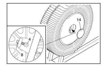
Pry the Access Cover (14) off the left side shield. Loosen the M8 Washer Nuts (4). To tighten the chain, turn the M6 Adjustment Nuts (8) clockwise; to loosen the chain, turn the Adjustment Nuts counterclockwise. Make sure that the fan is straight, tighten the Fan Nuts and reattach the Access Covers.
